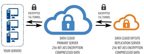
Data Cloud's backup agent is installed onto your servers and is connected to our Primary Backup Server via an encrypted SSL tunnel\*. Your data is then uploaded to our Primary Backup Server, and then securely replicated nightly to our Offsite Replication Server. Restores can be triggered remotely or physically, depending on the recovery scenario.
